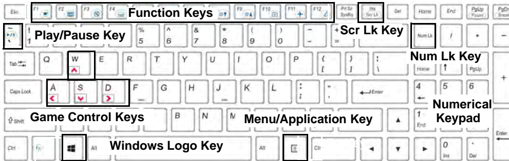
Figure 1 - 5 - Illuminated (White) LED Keyboard
