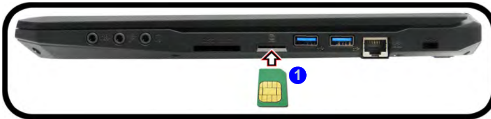
Figure 1 - 11 USIM Card Insertion
