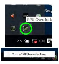
Overclocking should only be enabled when powered by a plugged-in adapter, and not on battery power. The Fan Speed will also automatically be set to overclock (do not adjust this fan speed setting if you have enabled GPU overclocking).
