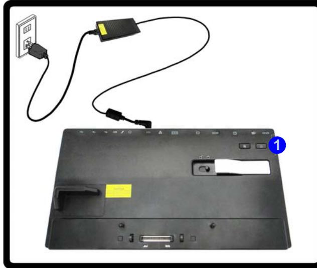
Figure E - 8 - Docking Station with AC/DC Adapter Plugged
