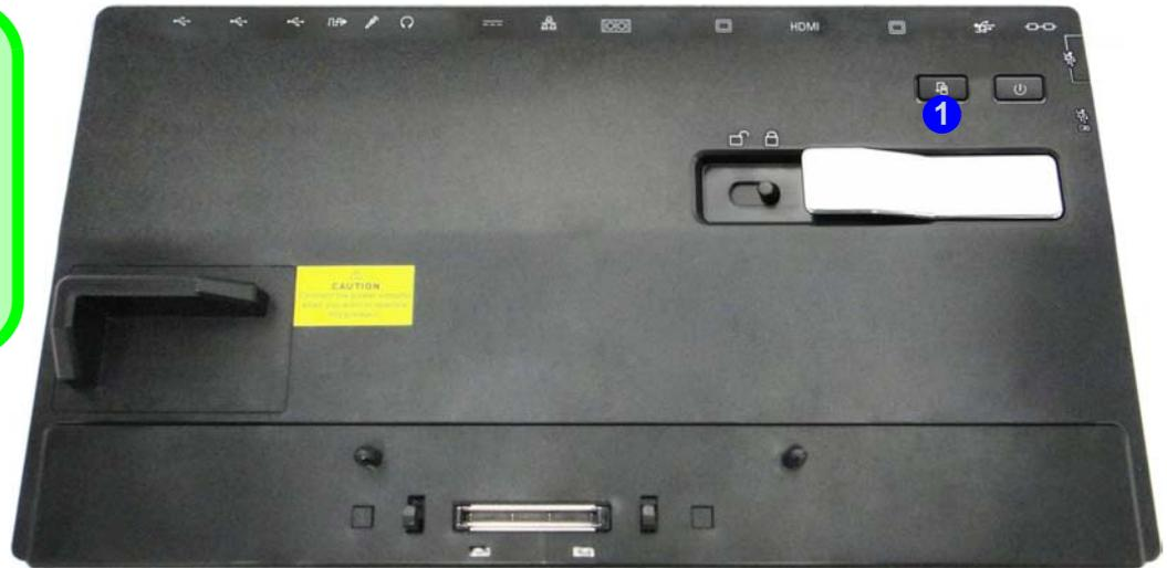
*Figure E - 13 - Front View (HDD Backup Hotkey)*
