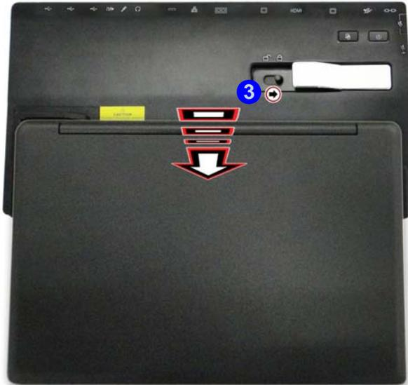
Figure E - 10 - Slide the Lock Switch
