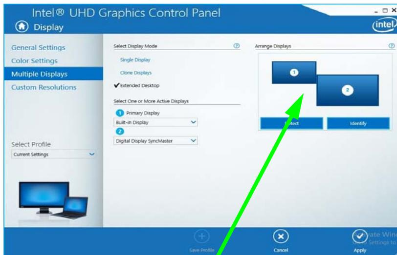
Click the appropriate monitor icon and drag it to match the physical arrangement you wish to use (e.g. the secondary display may be extended left/right/above/below the primary display).
