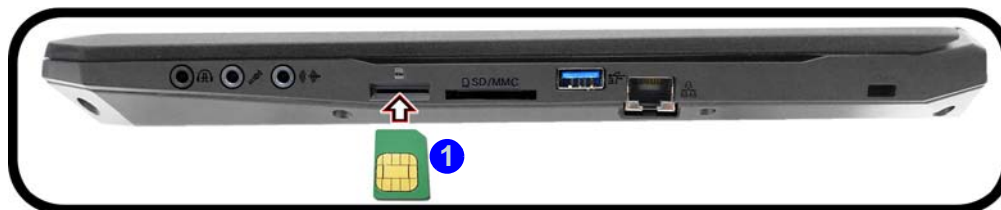
Figure 6 - 59 USIM Card Insertion
