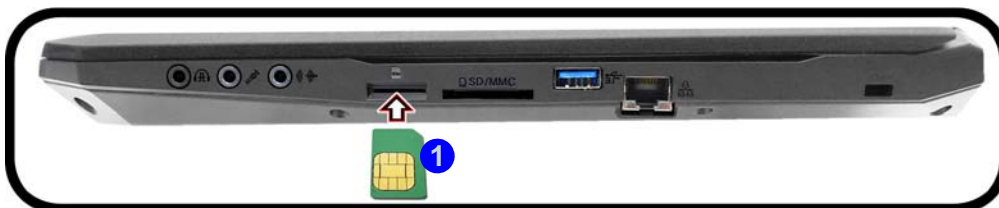
Figure 1 - 16 USIM Card Insertion
