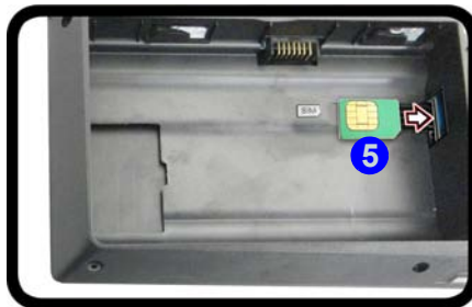
Figure 6 - 70 USIM Card & Battery Insertion
