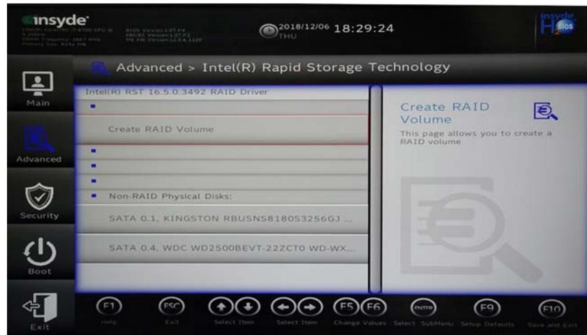
7. You can now setup your RAID volume using the installed SSDs.
