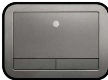
6. The fingerprint sensor in the Touchpad will flash, so repeatedly rest your finger on the sensor, and then lift it off until the setup is complete as instructed.
