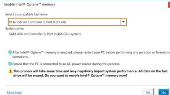
4. You will need to restart the computer after enabling **Optane**, and make sure the system is powered by the powered AC/DC adapter, and not by battery only.
