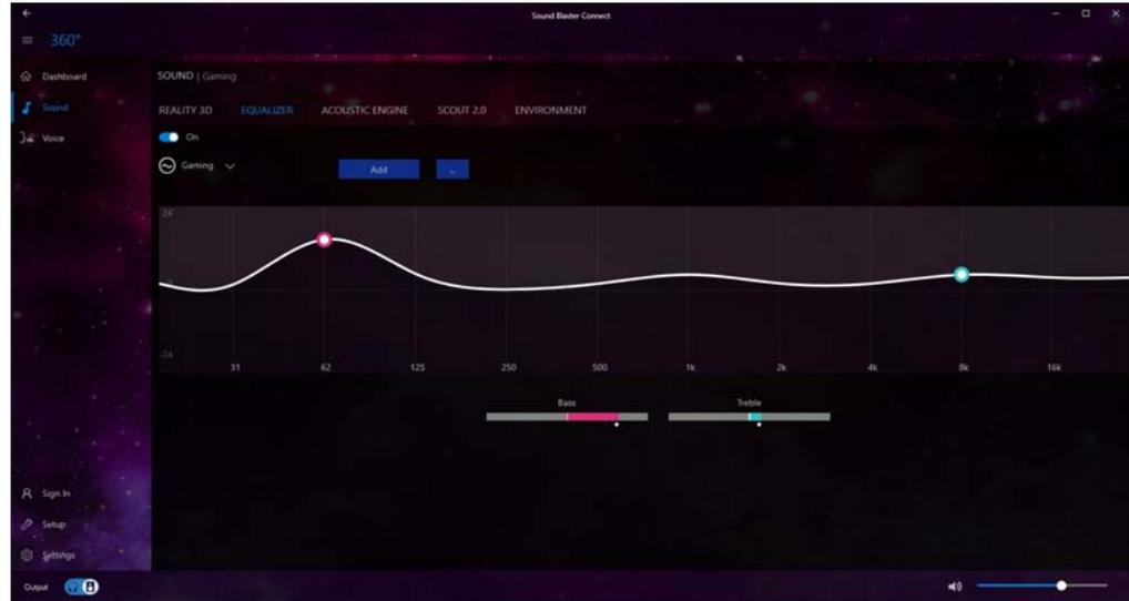
The **Acoustic Engine** offers a suite of playback technologies to enhance sound. Each playback technology has an **On/Off button** to allow you to enable/disable it, and most controls feature a dial to adjust the levels.
