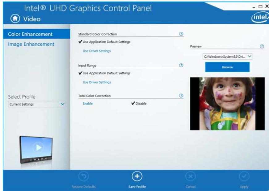
Click the **Video** menu at the top of the screen to display the sub-menus. The **Image Enhancement** menu allows you to adjust the **Sharpness**, **Skin Tone Enhancement**, **Noise Reduction**, **Contrast Enhancement** and **Film Mode Detection**. Click **Apply** to save changes.
